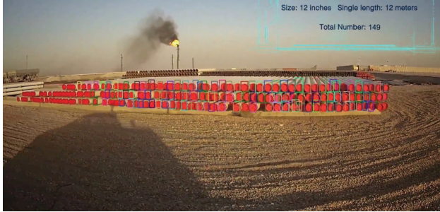
Fig. 6. Real-Time Detection and Counting Result
